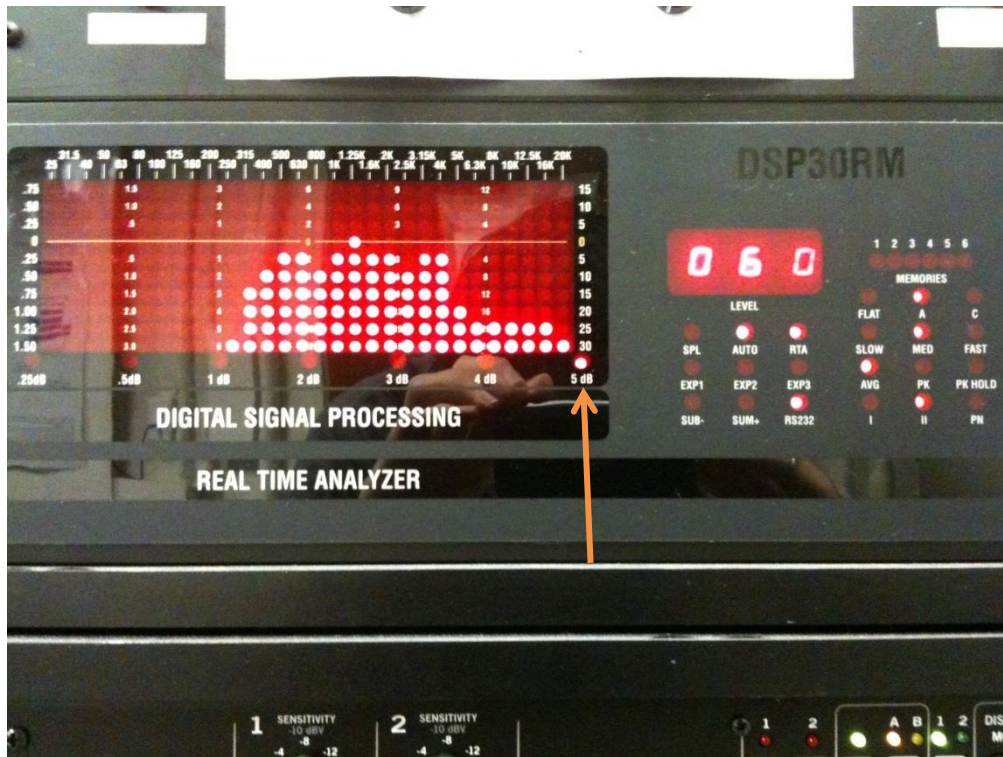
Figure D-2. Real time spectrum analysis of pink noise in Chamber 1.
